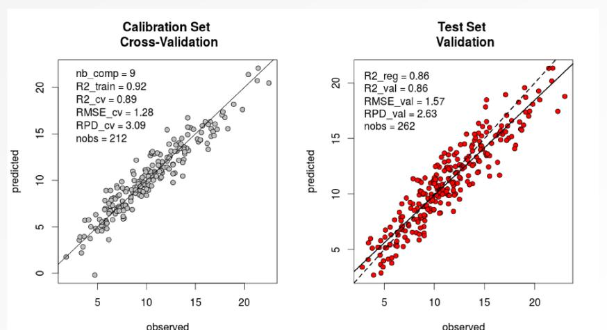
**Fig. 4 :** NIRS model for STB amount in scots pine wood following an automatic selection of wavenumbers.
