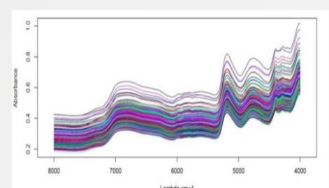
**Fig. 2 :** Raw spectra from Scots pine heartwood surface measurements by NIRS.
